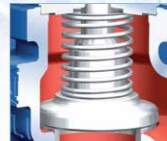
Maximum cost effectiveness: "Two-in-One" (screw-down non-return plug with resetting spring provides additional function as a check valve with shut-off feature)
